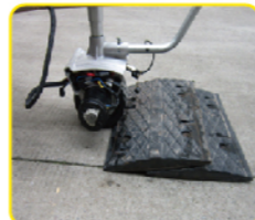
Max pulling incline is 7°
