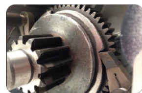
Double-lock brake system
